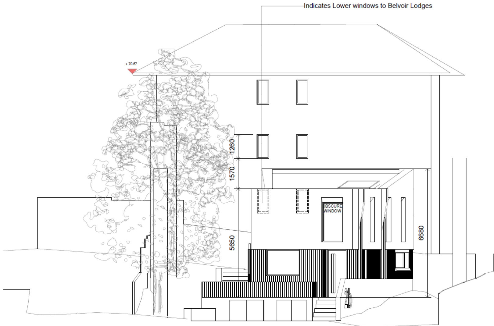
Proposed front elevation of new house
